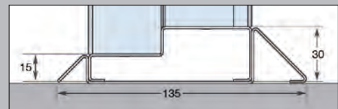
Optional 30mm threshold with ramped adjustable baseplate
