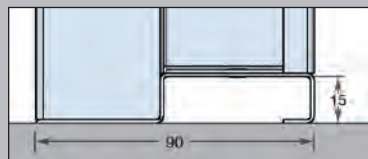
Standard 15mm low profile threshold
